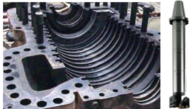
Typical turbine housing
